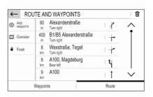
To display a turning manoeuvre on the map, touch the turn arrow icon next to the desired list entry. The map jumps to the respective location on the map.
